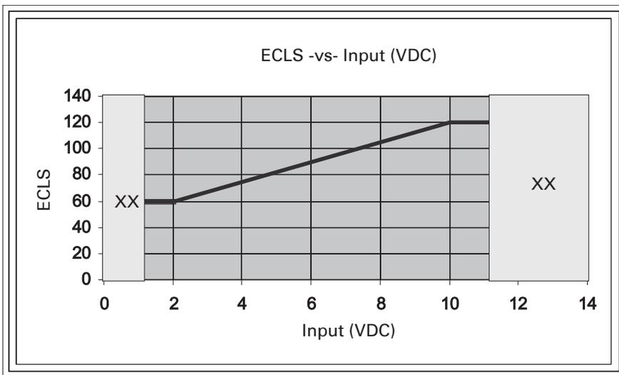
For input signals beyond the 2-10VDC or 4-20mA range, the end of range value is used. For example, if the customer inputs 21 mA, the ECLS limits it self to the corresponding 20 mA ECLS.
